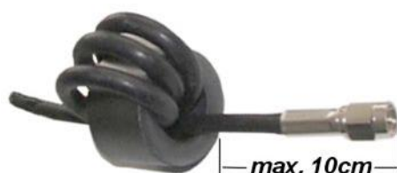
Figure 10: Antenna cable with EMV ferrite core
