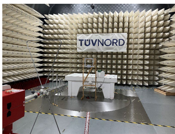
Test setup: SAC 30 MHz to 1 GHz
