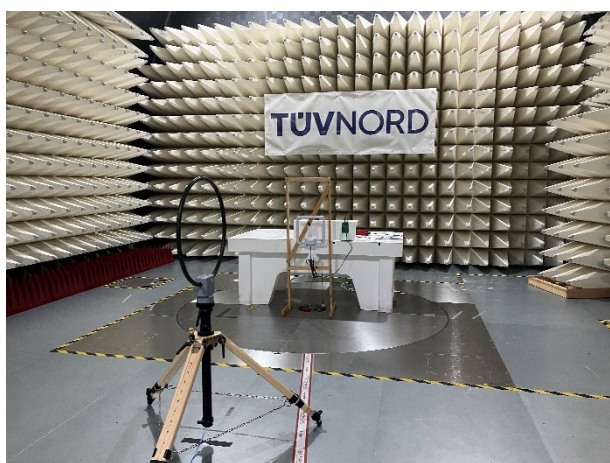
Test setup: SAC 9 kHz to 30 MHz
