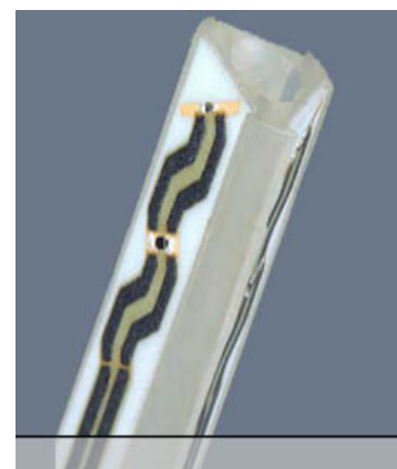
ET3DV6 E-Field Probe
