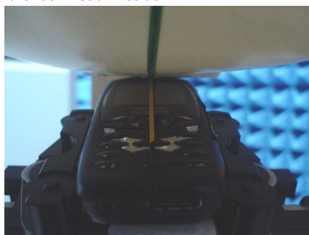
Fig.4 Right Head Section / Ear-Tilt Position(15°)
