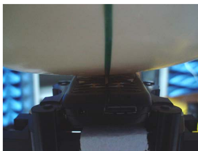
Fig.5 Left Head Section / Cheek-Touch Position
