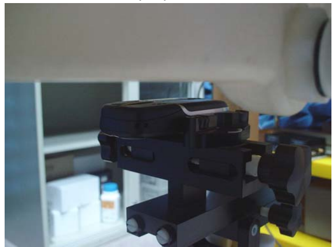
Fig.7 Body Position (Testing in GPRS mode)
