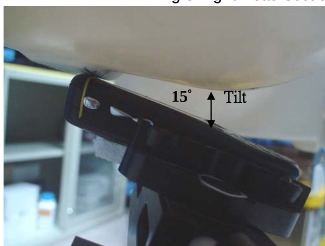
Fig.4 Right Head Section / Ear-Tilt Position(15°)
