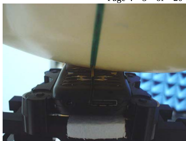
Fig.3 Right Head Section / Cheek-Touch Position
