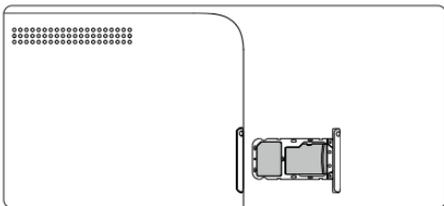
2. Insert/remove the SIM and microSD card.
