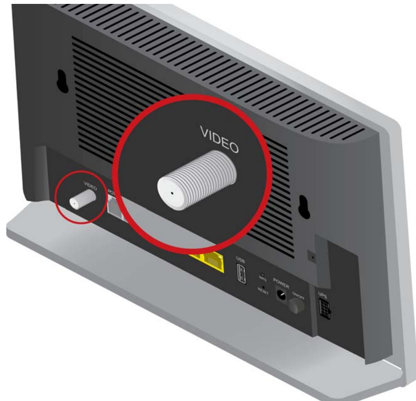
Figure 21: The coaxial video port.
