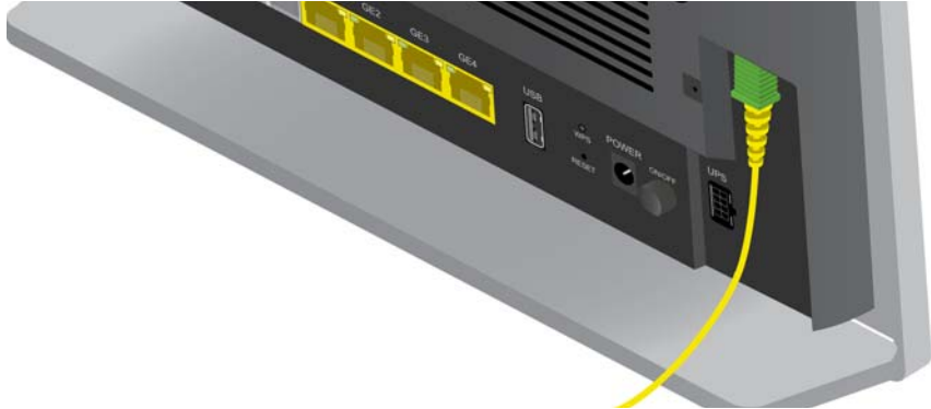
Figure 16: zNID-GPON-27xx models use SC/APC connector (green)
