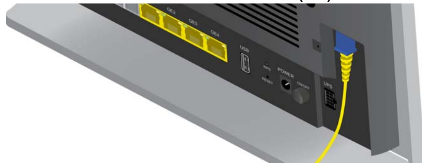
Figure 17: zNID-GE-27xx models use SC/UPC connector (blue)
