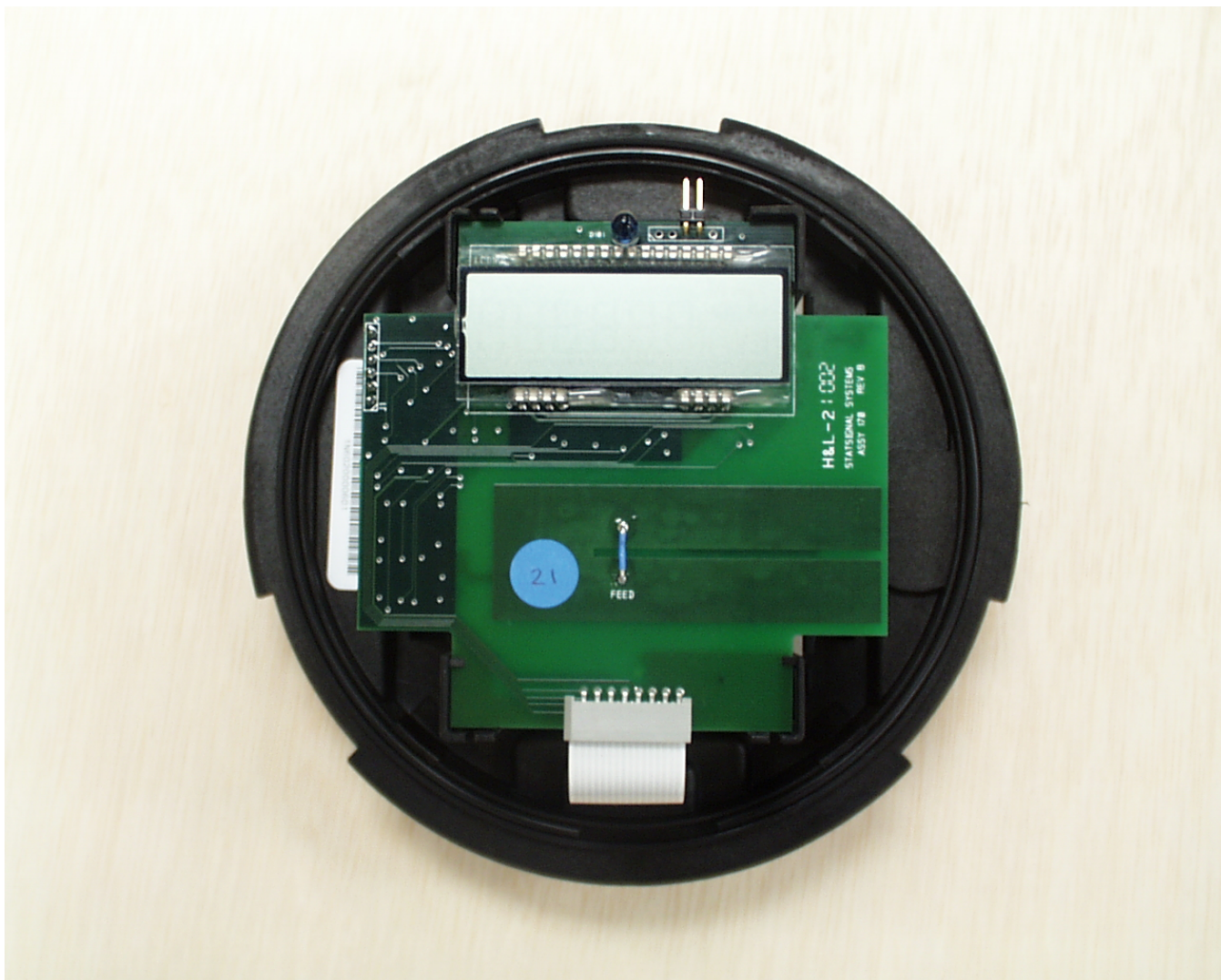
Internal Photograph 3: Top view of transmitter circuit board (assembled)
