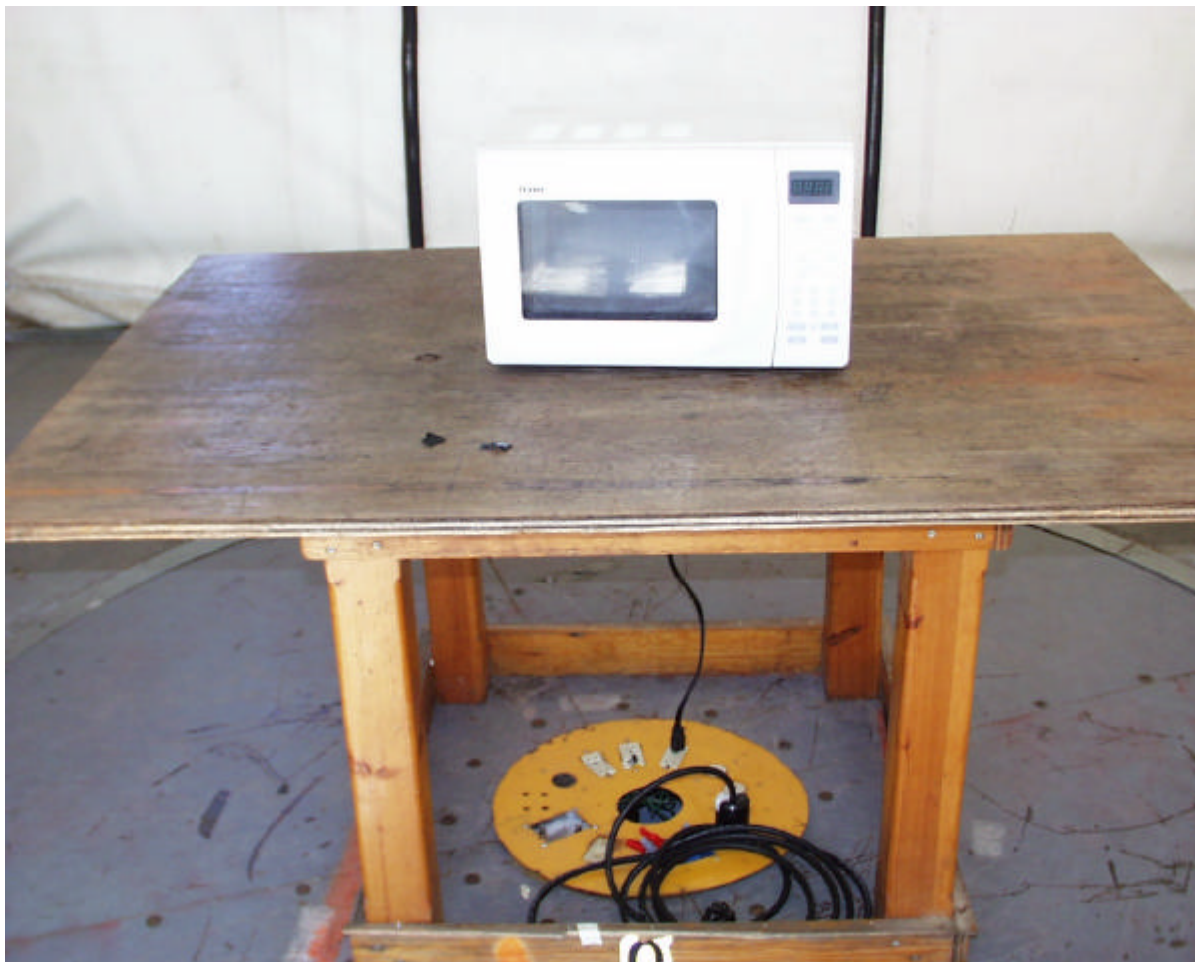
RADIATED TEST SETUP BELOW 1GHz (FRONT SIDE)
