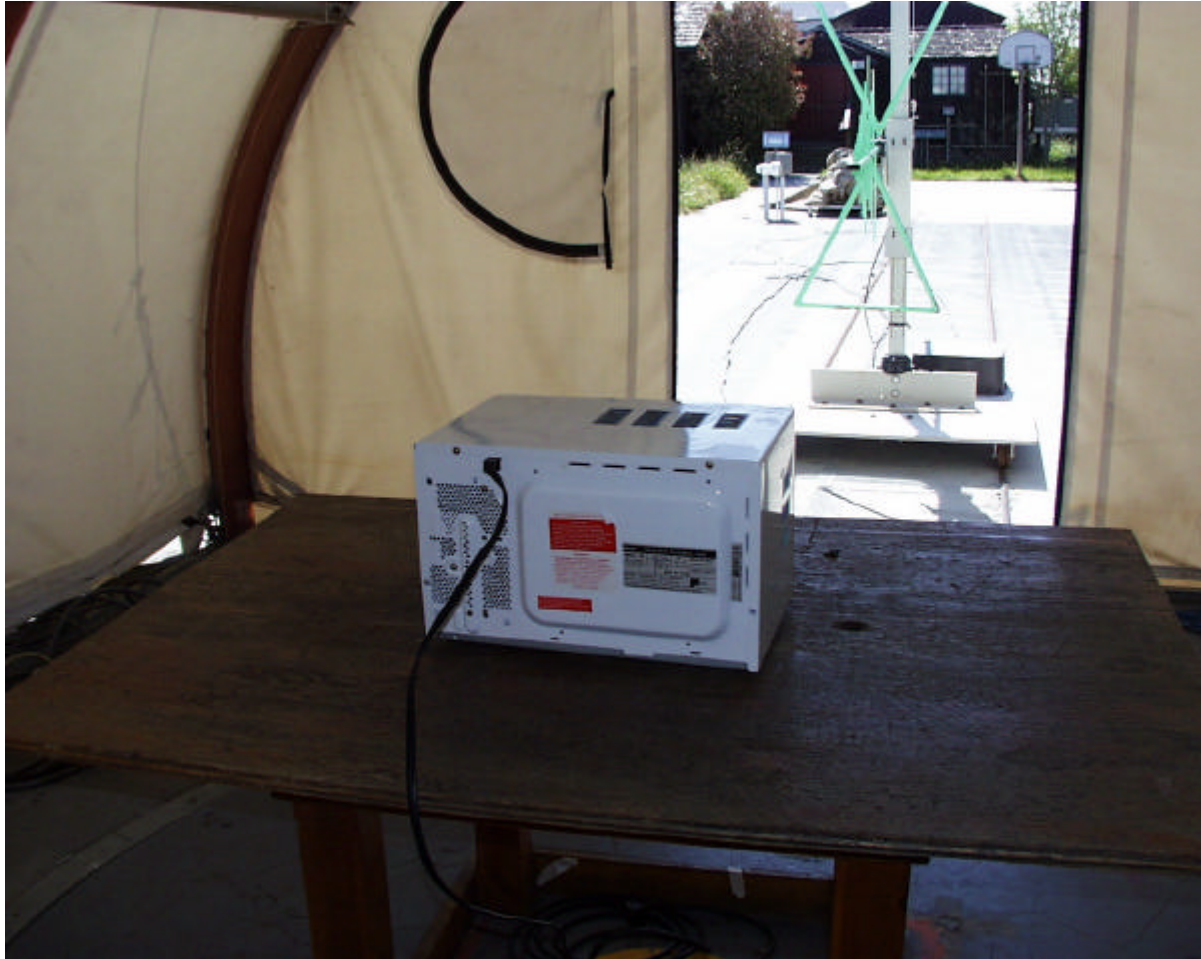
RADIATED TEST SETUP BELOW 1GHz (BACK SIDE)
