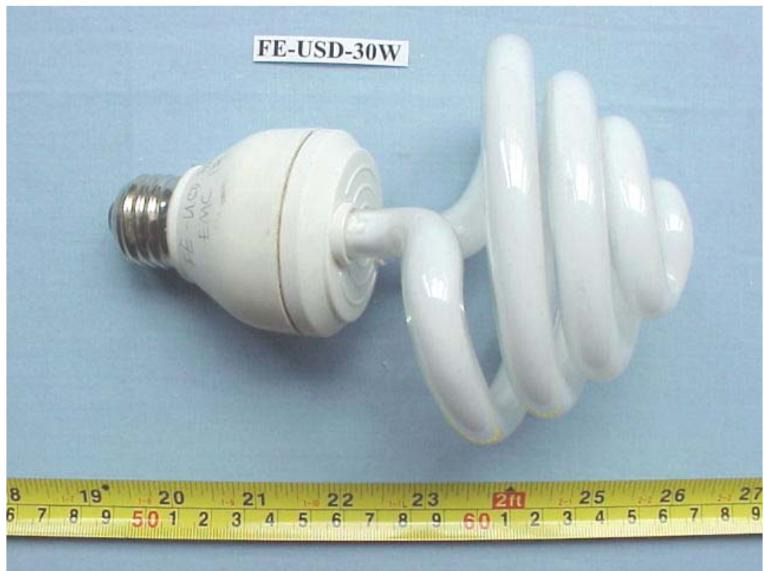
FIGURE 13 ENERGY SAVING LAMP (M/N: FE-USD-30W) GENERAL APPEARANCE
