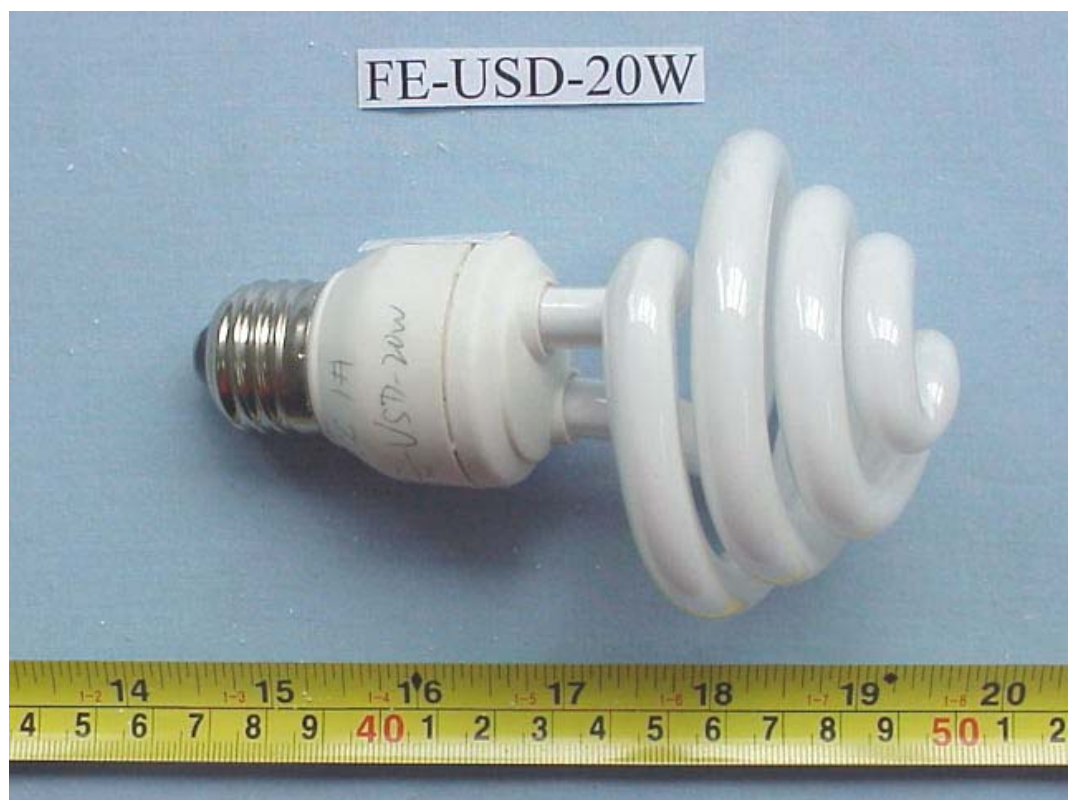
FIGURE 10 ENERGY SAVING LAMP (M/N: FE-USD-20W) GENERAL APPEARANCE
