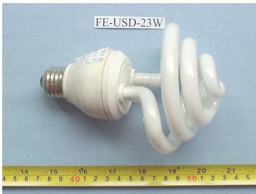
FIGURE 11 ENERGY SAVING LAMP (M/N: FE-USD-23W) GENERAL APPEARANCE
