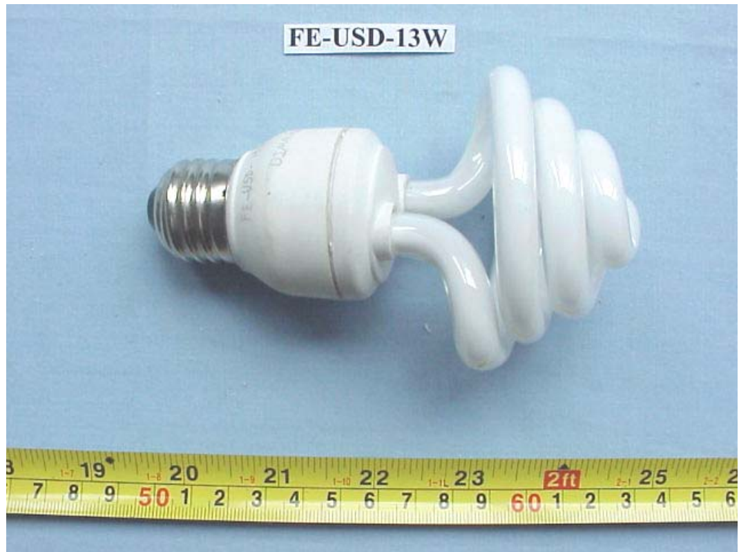
FIGURE 7 ENERGY SAVING LAMP (M/N: FE-USD-13W) GENERAL APPEARANCE
