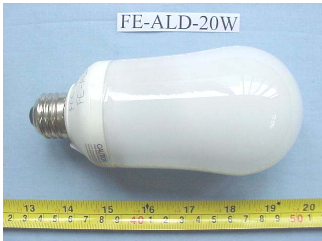
FIGURE 42 ENERGY SAVING LAMP (M/N: FE-ALD-20W) GENERAL APPEARANCE
