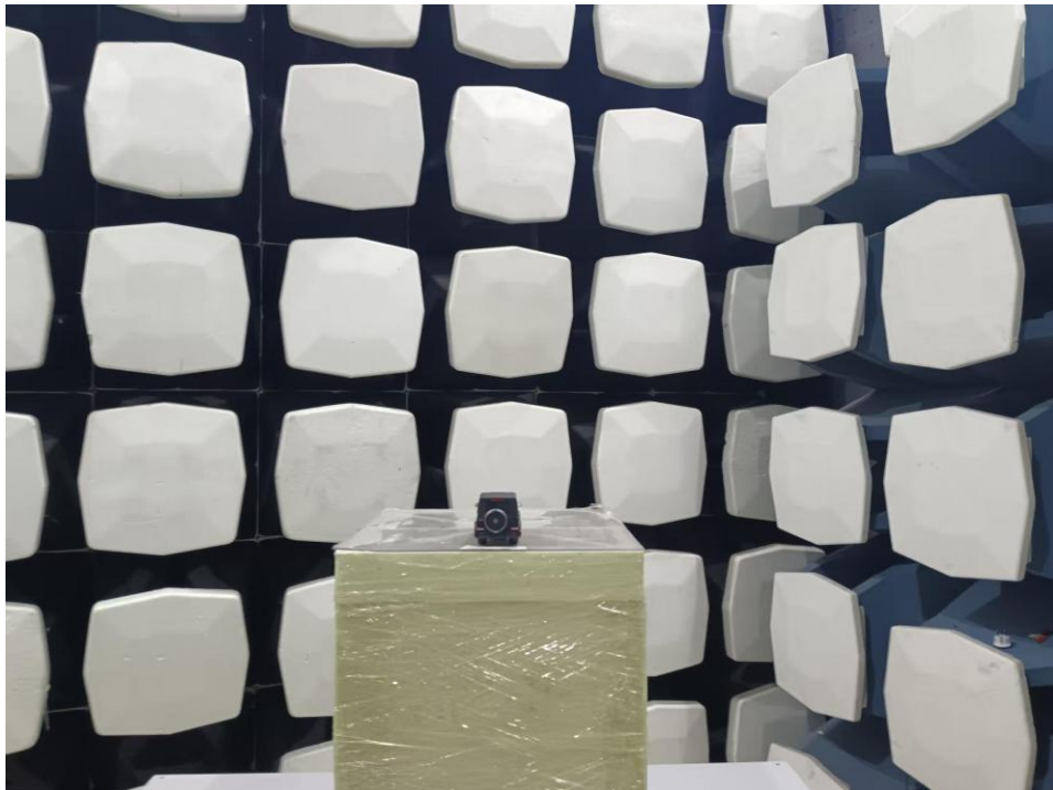
18GHz-25GHz (EUT was placed in the centre of the turntable)
