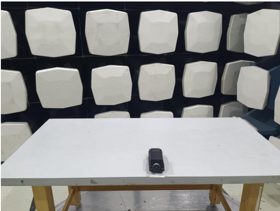
9KHz-30MHz (EUT was placed in the centre of the turntable)
