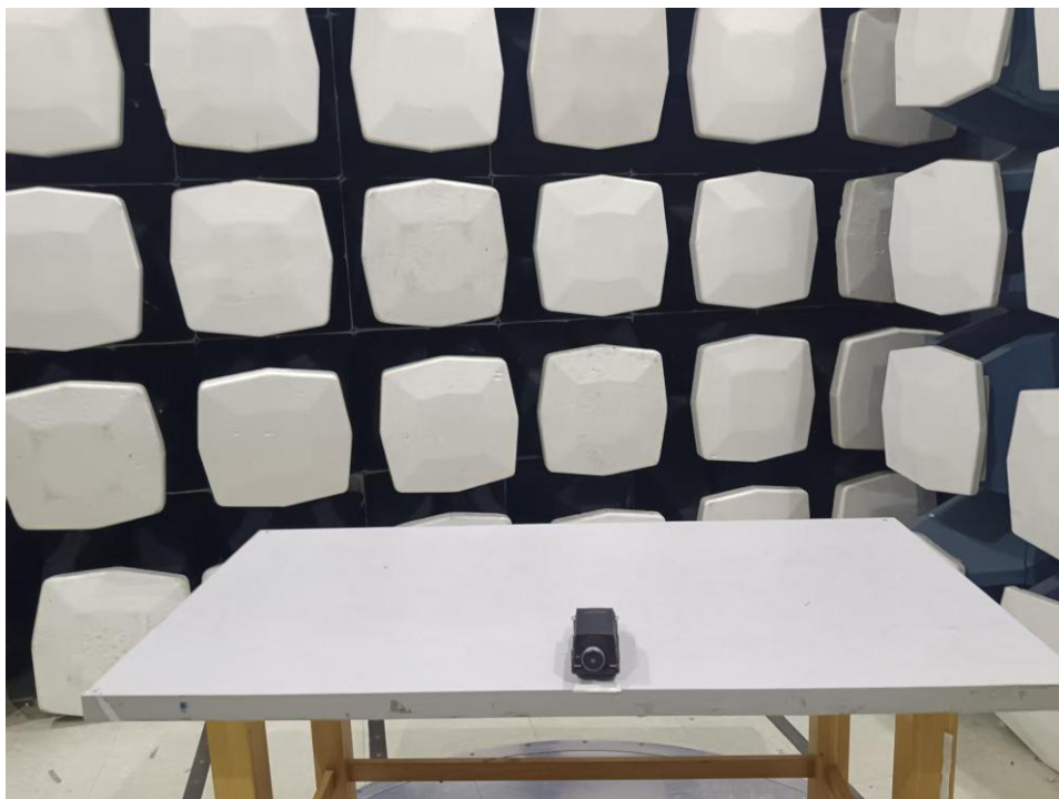
30MHz-1GHz (EUT was placed in the centre of the turntable)
