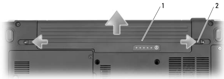
1 battery 2 battery release latch (2)
