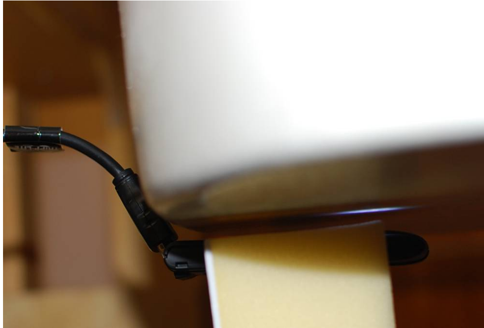
Figure 18-1 SAR Test Setup Photo 1, Horizontal-Down
