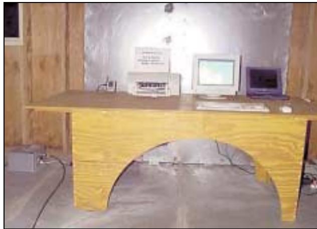
Mains Conducted Emissions Test Setup - Front View
