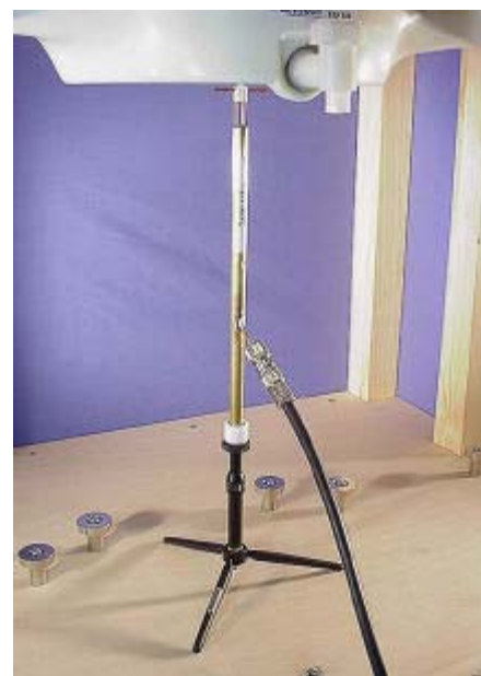
2450MHz Dipole Validation Setup
