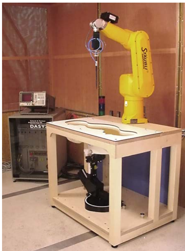
DASY3 SAR Measurement System with SAM phantom
