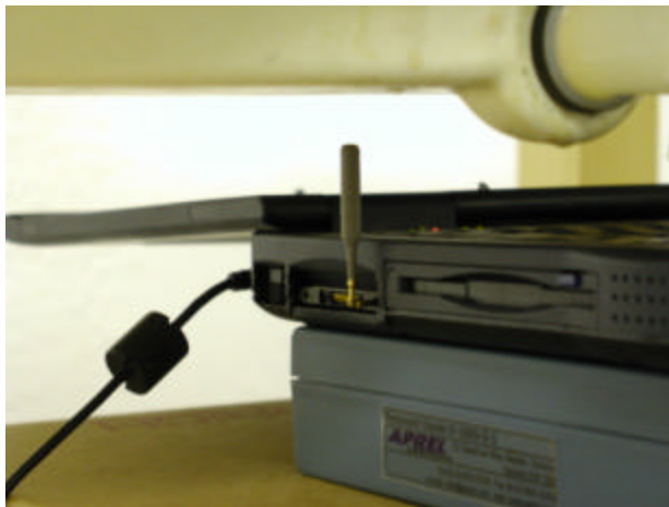
Photo 4: HP T18.033.C.00 keyboard facing with phantom, antenna perpendicular to laptop
