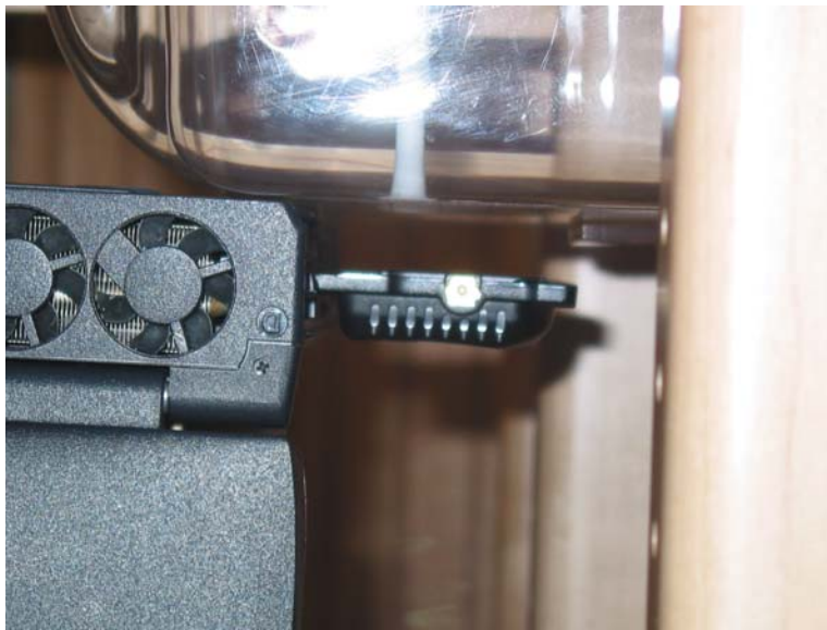
Figure 1 – Dell Internal Antenna Touch Position
