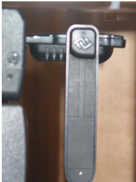
Figure 2 – Dell External Antenna Touch Position
