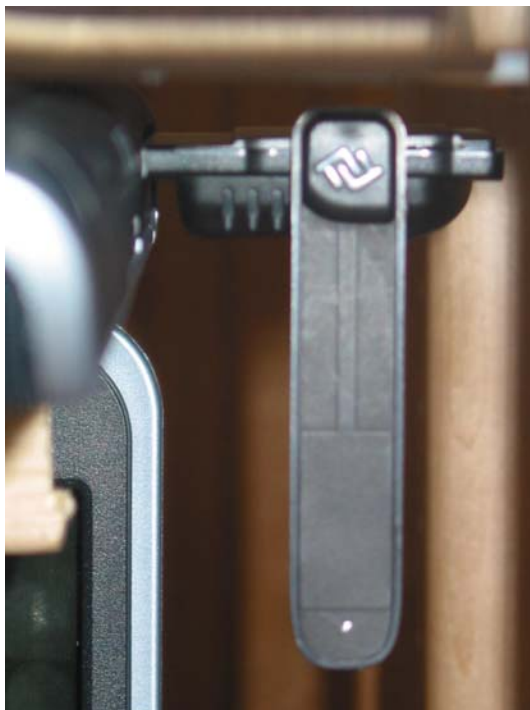
Figure 4 – HP External Antenna Touch Position
