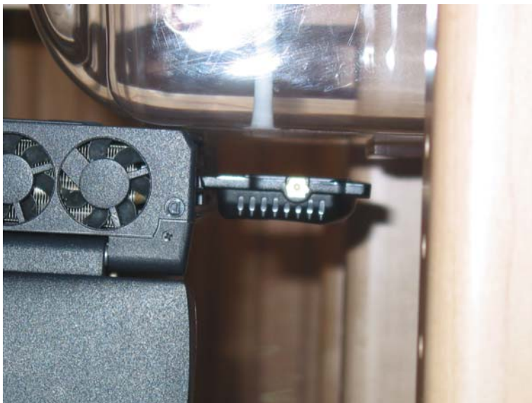
Figure 1 – Dell Internal Antenna Touch Position
