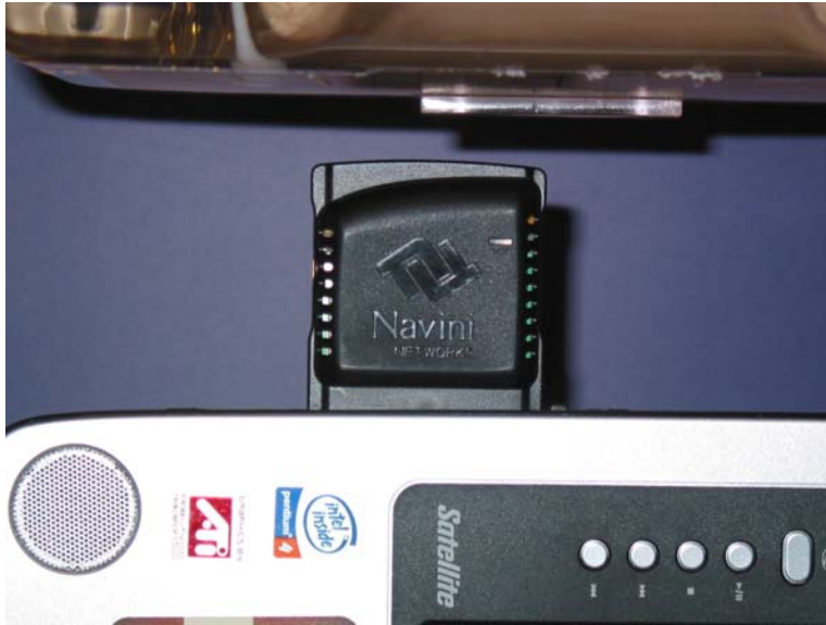
Figure 7 – Toshiba Internal Antenna 15 mm Position
