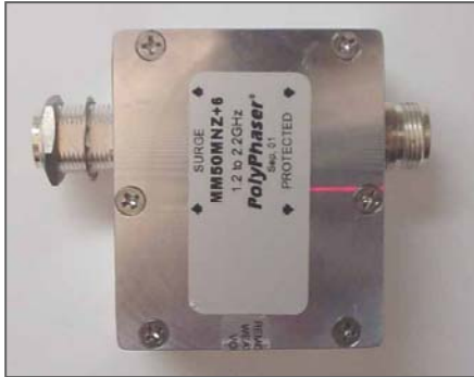
Figure 9: GPS Cable Surge Protector
