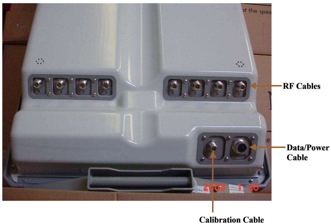
Figure 16: Panel Cable Routing
