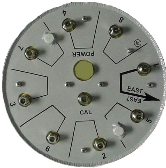
Figure 29: Omni Antenna Elements
