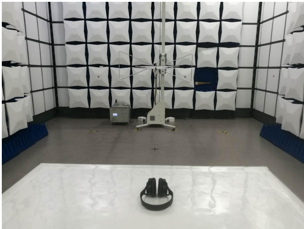
FCC RADIATED EMISSION TEST SETUP
