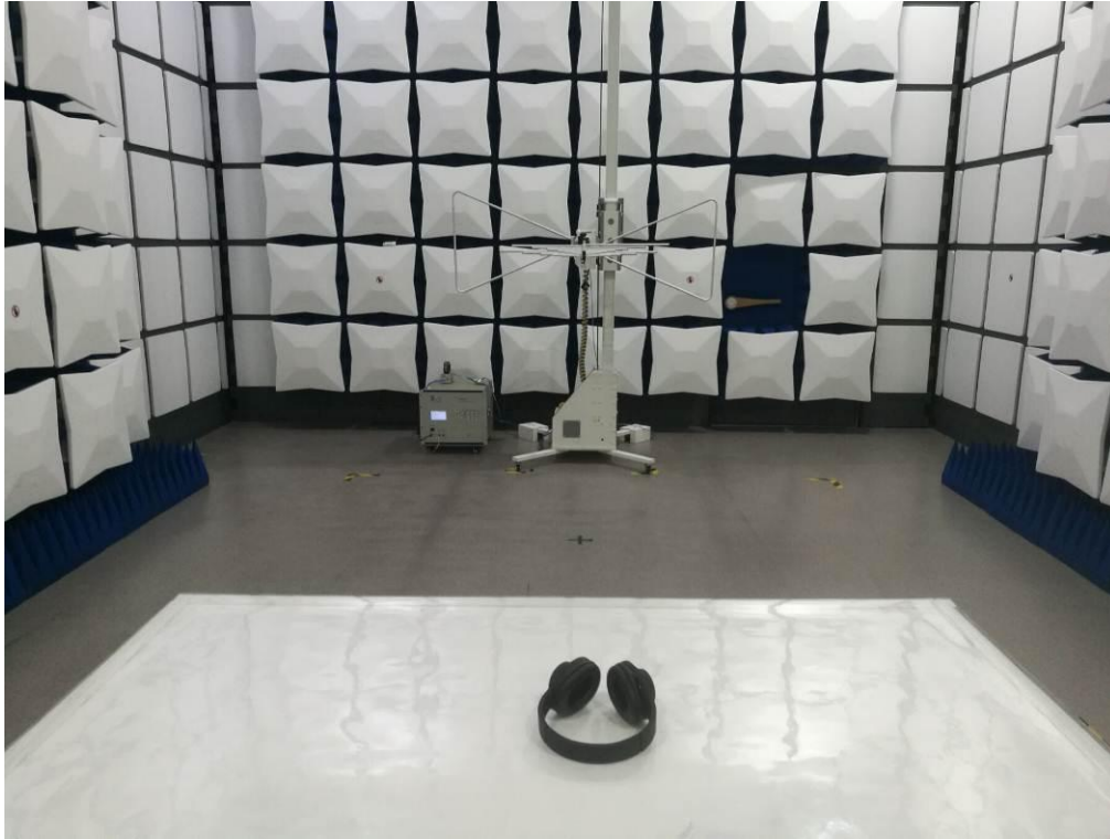
FCC RADIATED EMISSION TEST SETUP
