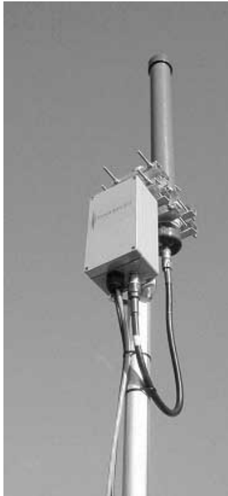
Figure 3-1: Omnidirectional transmitter and antenna.
