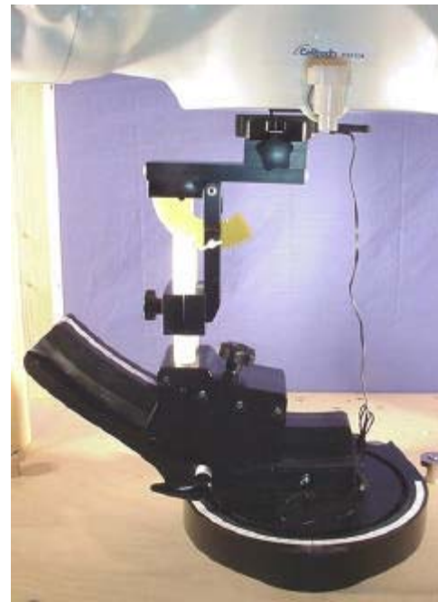
Body-worn SAR Test Setup
