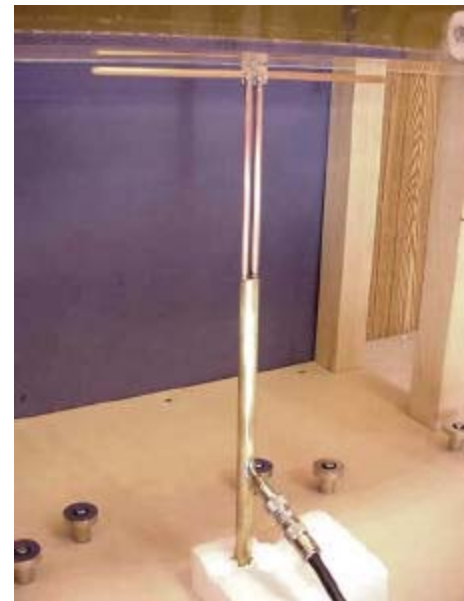
450MHz Dipole Validation Setup
