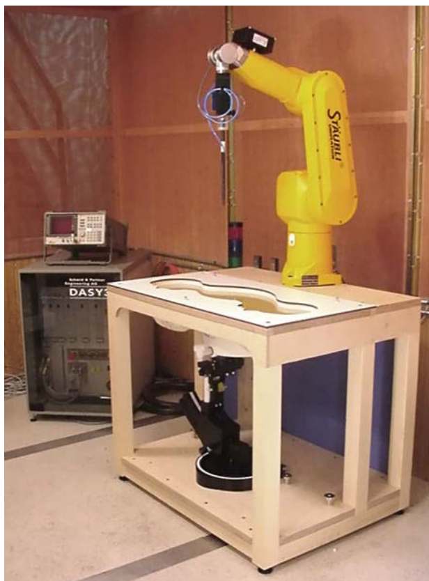
DASY3 SAR Measurement System with SAM Phantom
