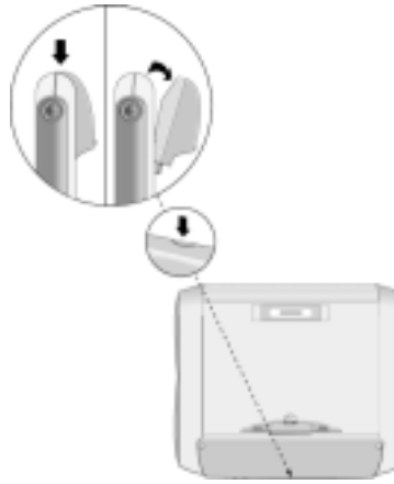
Figure - Replacing Main Battery
