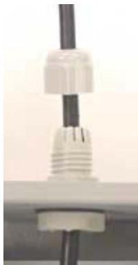
Figure 5-13 – Securing the PIM's Antenna NEMA Gland
