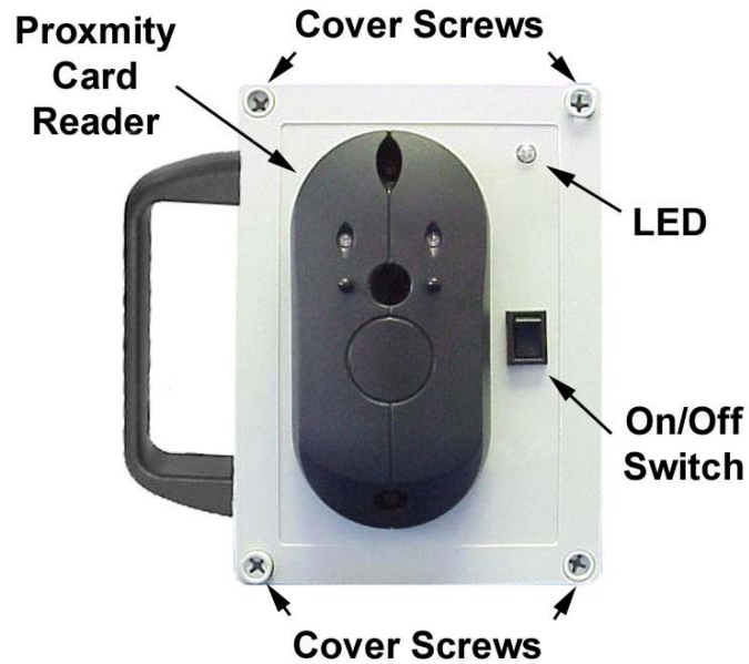
Figure 8-1 – Wireless Portable Reader (WPR) with Proximity Reader
