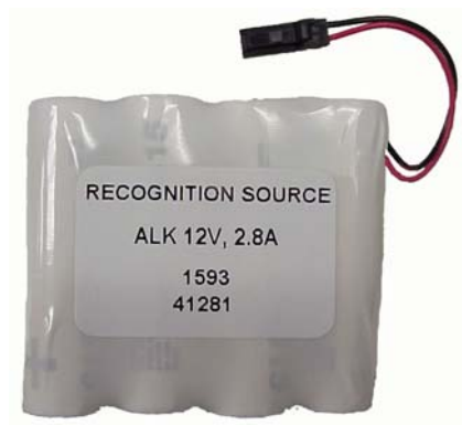
Figure 6-2 – WISI Battery Pack
