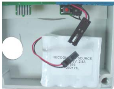
Figure 9-4 – Removing the Used Battery Pack
