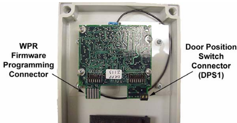
Figure 8-2 – WPR PCB Connectors
