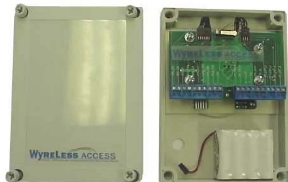
Figure 6-3 – Control Transceiver with Cover Removed
