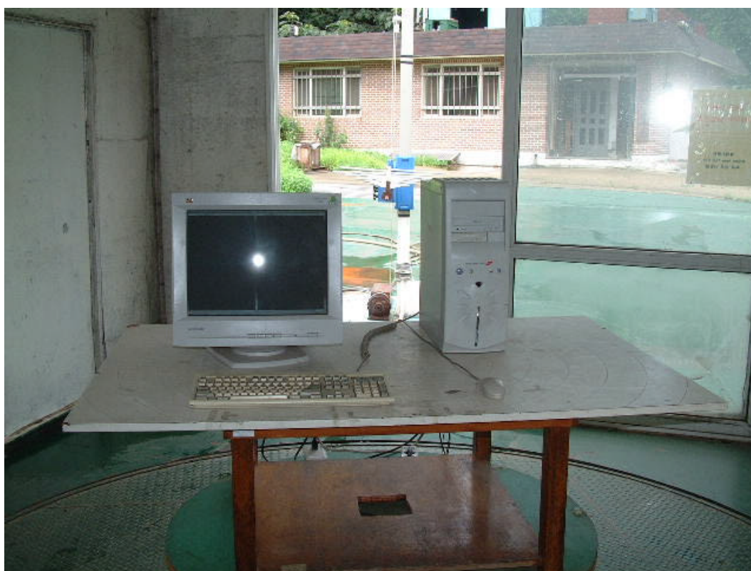
RADIATED EMISSION SETUP PHOTOGRAPH - FRONT VIEW ( 300- 1000 MHz )
