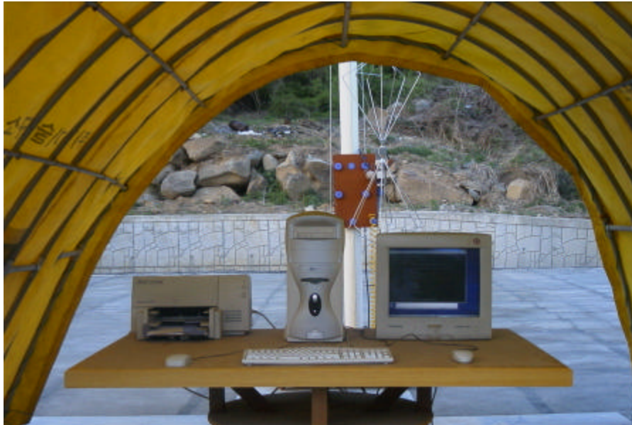
Photograph 1 : Setup for radiated Emissions
