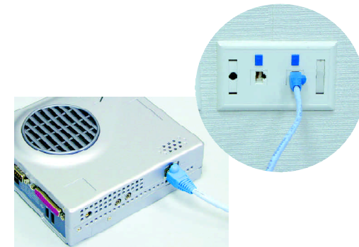
Figure 3-6 Connecting to the LAN
