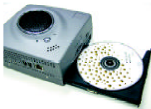
Figure 3-4c Removing the Compact Disc Inside
