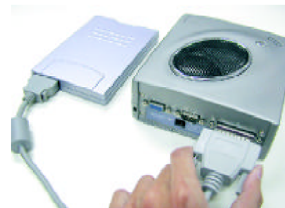
Figure 3-2 Connecting the External FDD via the Parallel Port
