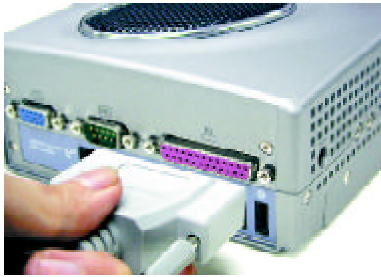
Figure 4-2 Connecting a Printer
