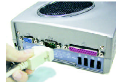
Figure 4-1 Connecting a Serial Device
