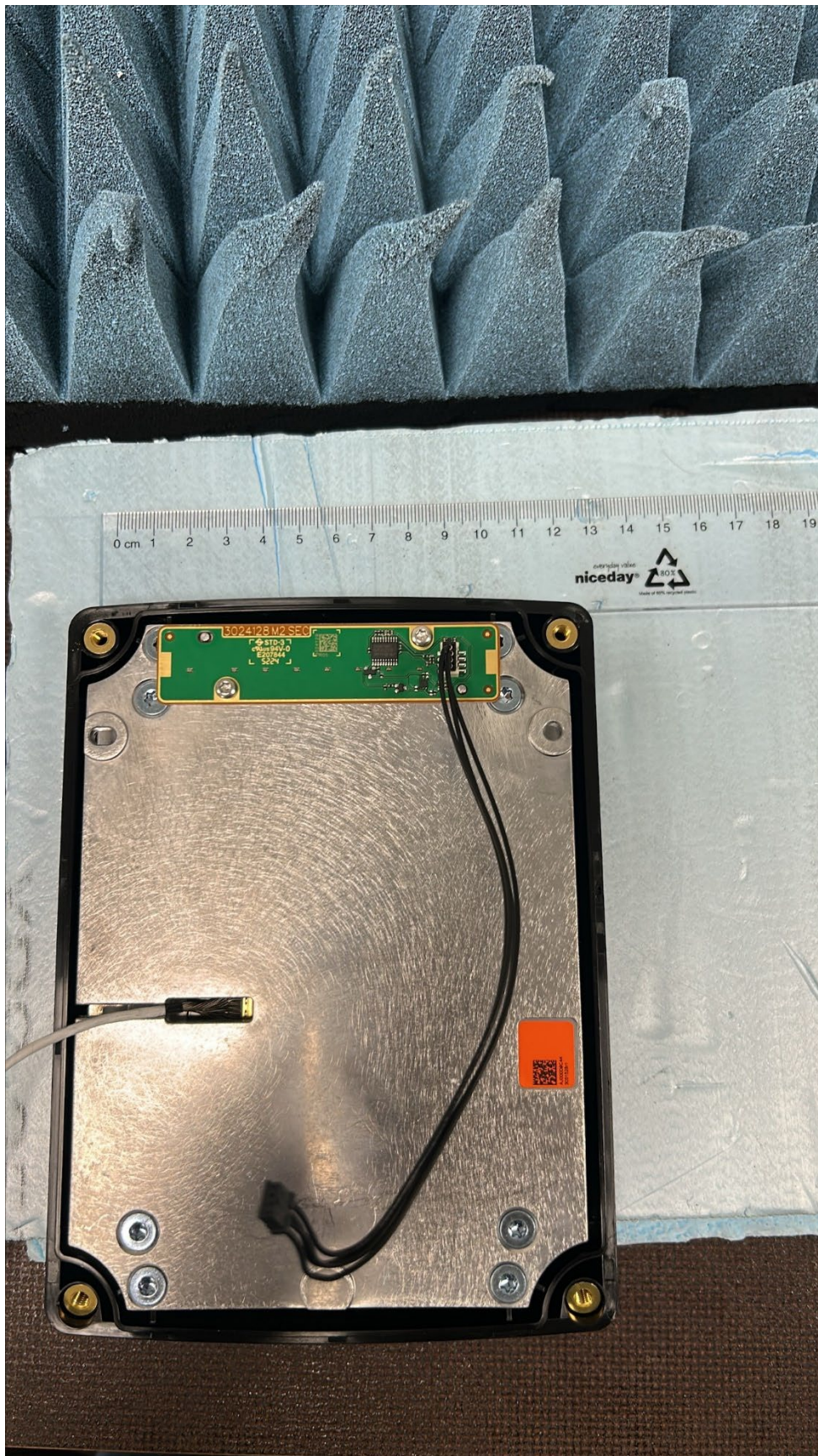
Figure 4: RF module back, with shield
