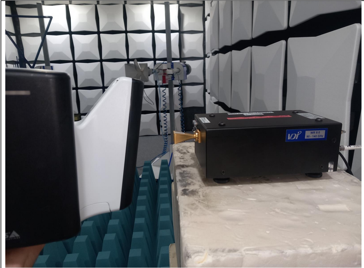
Test setup: Radiated measurements 90GHz to 140 GHz (0.1 m) Manuel exploratory over whole sphere of EUT
