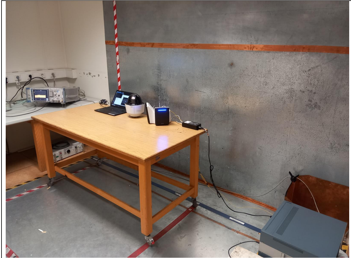
Test setup: AC-Conducted measurements
