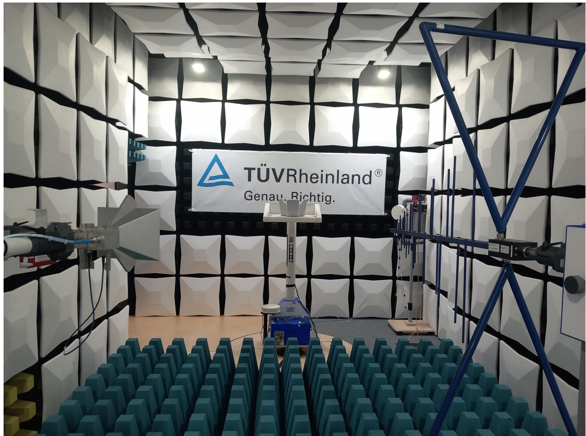
Test Setup: Radiated Measurements (1 GHz to 40 GHz)
