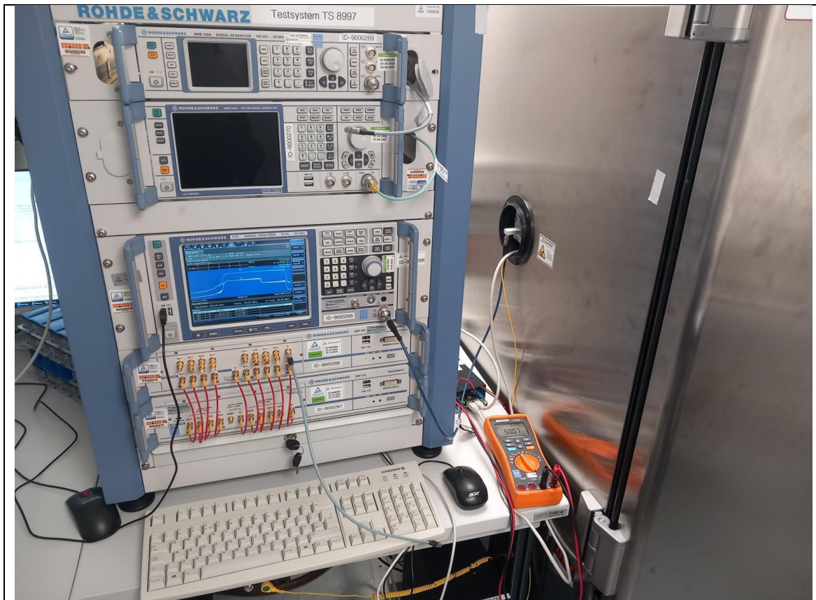
Test setup: Conducted measurements in normal and extreme conditions Measurement-Equipment-Side
