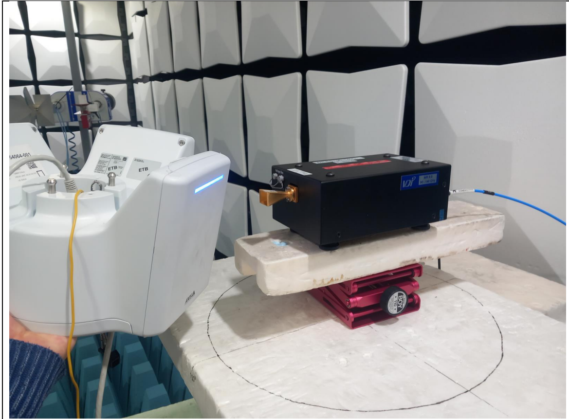
Test setup: Radiated measurements 60GHz to 140 GHz (0.1 m) Manuel exploratory over whole sphere of EUT
