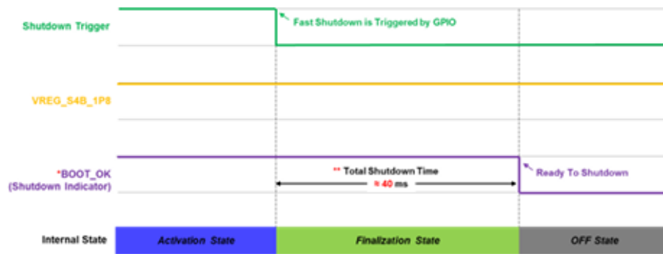
Figure 8: Fast Shutdown by GPIO (*SHDNIND Enable, Optional)
