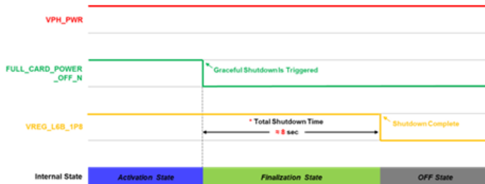
Figure 6: Graceful Shutdown by FULL_CARD_POWER_OFF_N
