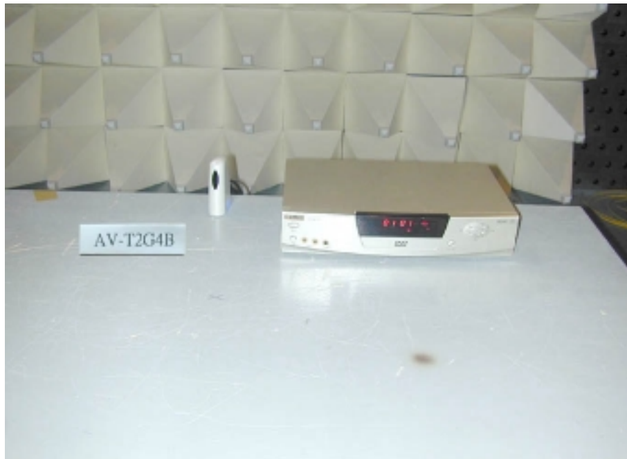
Photo 2: Radiated Emission Test Set-up (rear)
