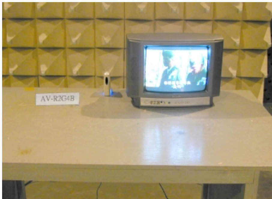
Photo 2: Spurious Emission Test Set-up (rear)
