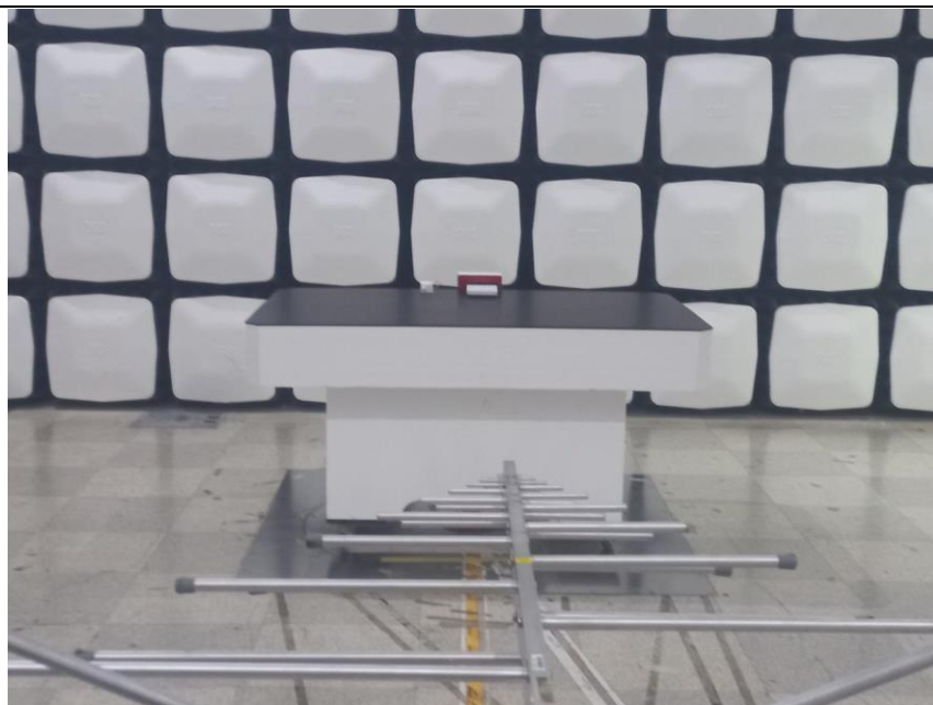
[Rear view of Radiated Emission (below 1GHz)]
