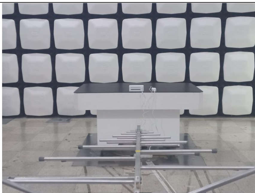
[Rear view of Radiated Emission (below 1GHz)]
