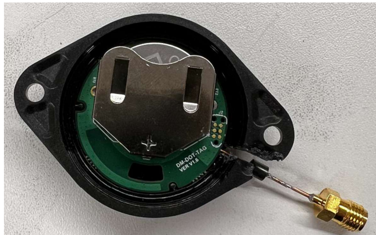
DUT with the implemented F-antenna and cabling setup
