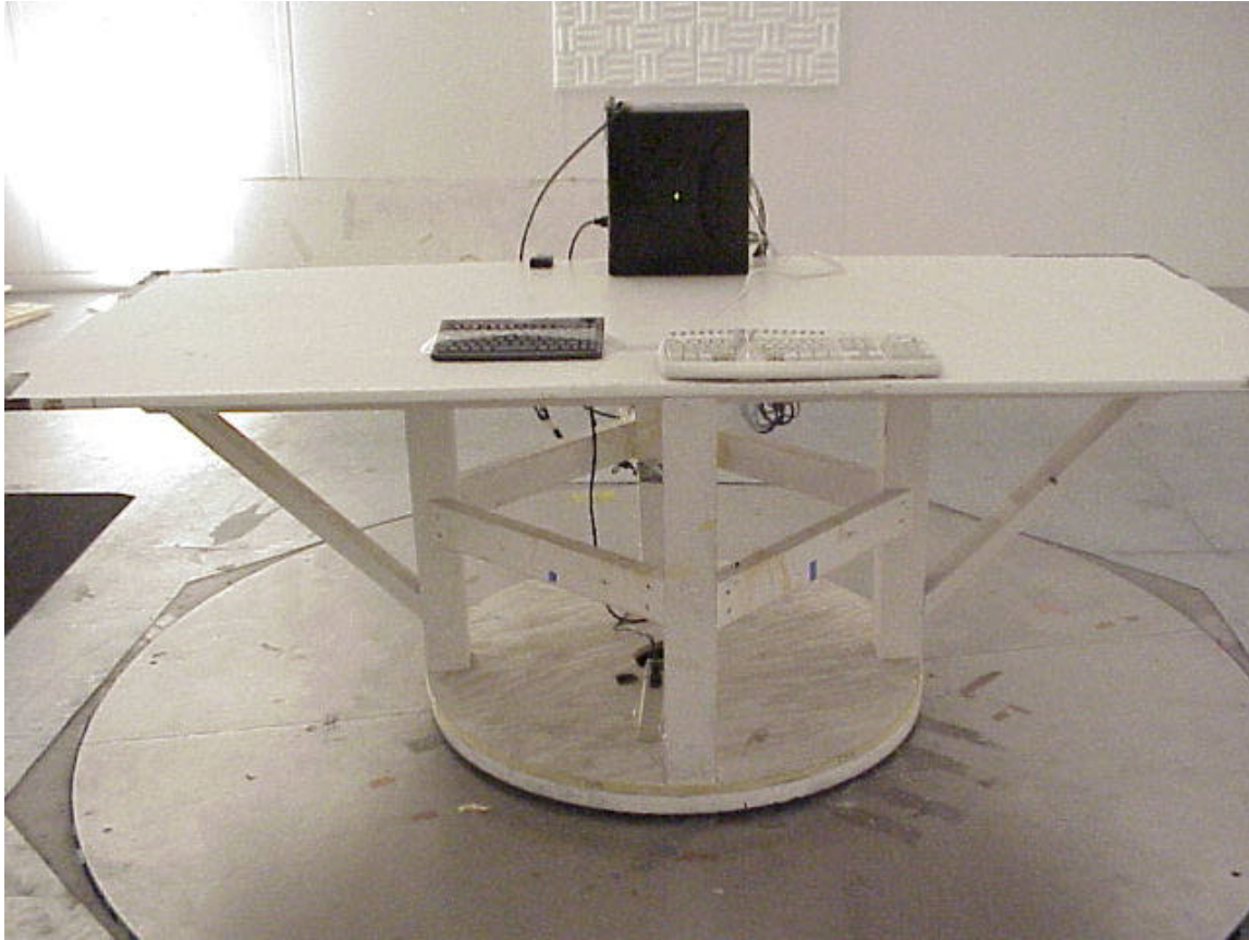
Worst Case Radiated Emissions Test Configuration
