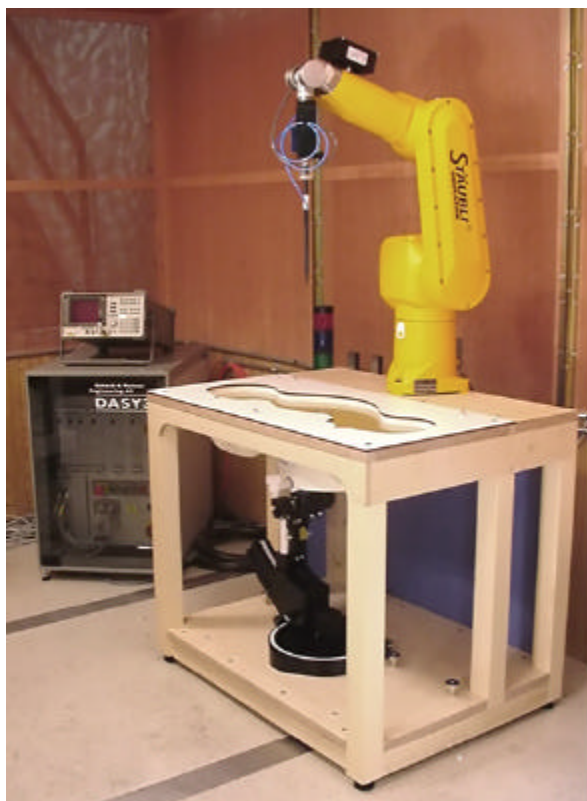
DASY3 SAR Measurement System with SAM phantom
