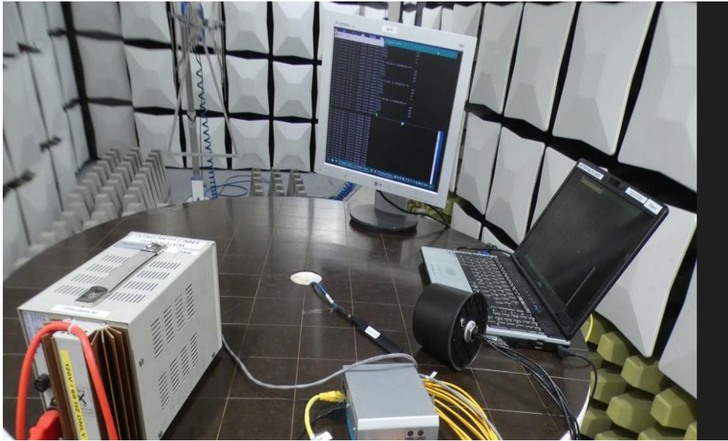
Photo 3: Test setup for radiated measurements FCC15b, 18 GHz – 40 GHz
