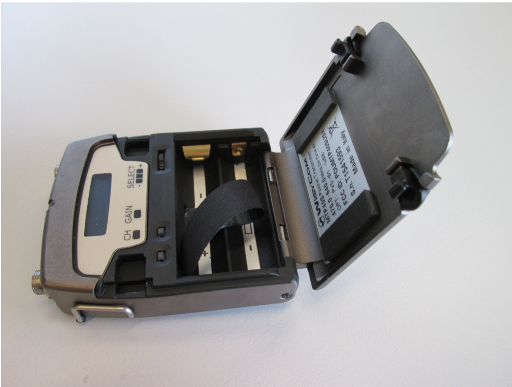
Exemplary photo of EUT #T1541593, battery case view
