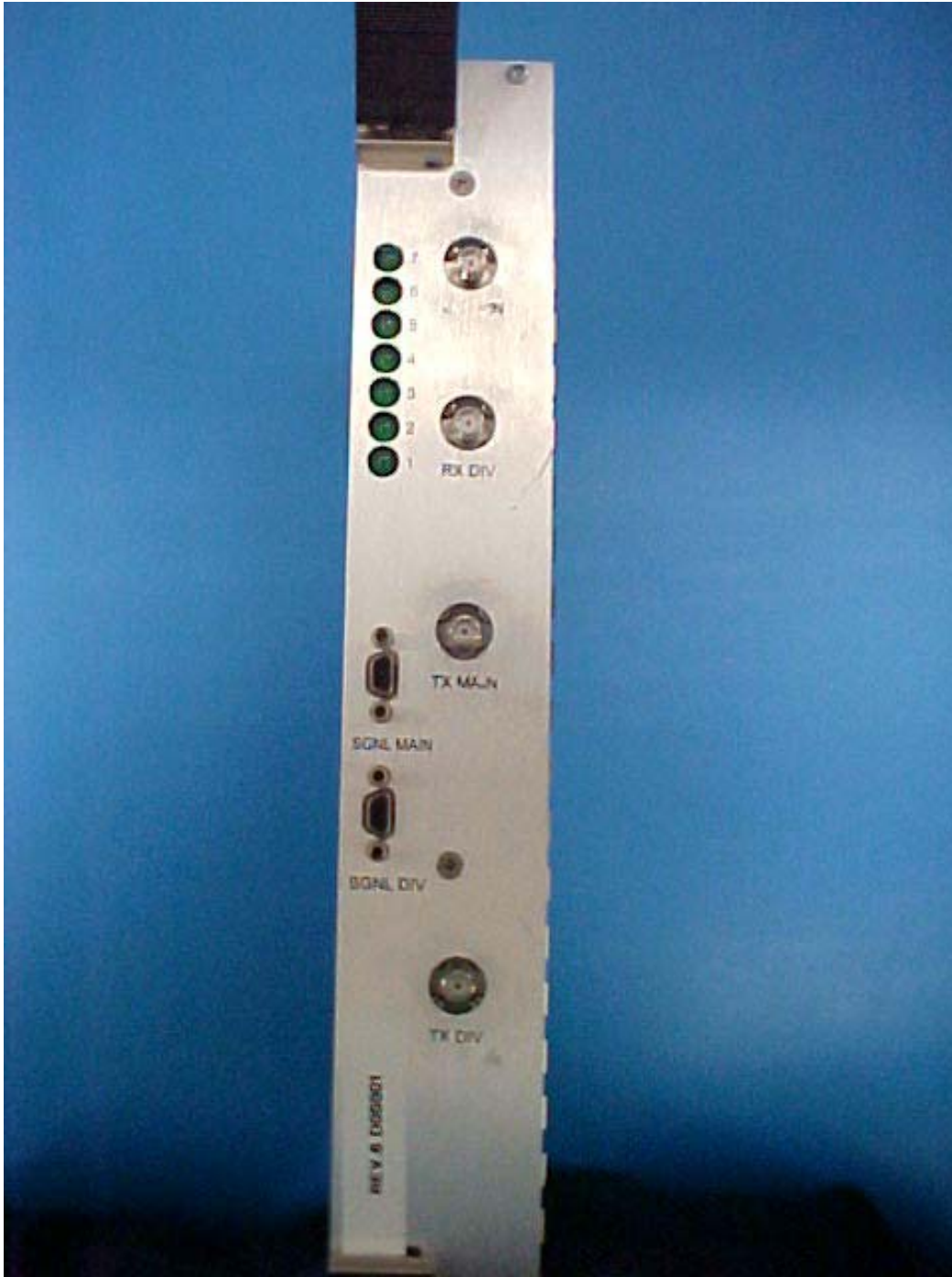
Front side of the IF card (Only the front side was taken since the card requires a rack to shield the board)
