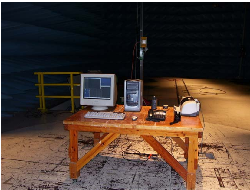
Photograph 6. Radiated Emission Limits Test Setup, 1 GHz to 2 GHz, Front View
