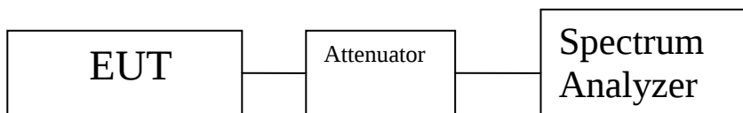
Figure 4. Block Diagram of Spurious Emissions at Antenna Terminals Test Setup
