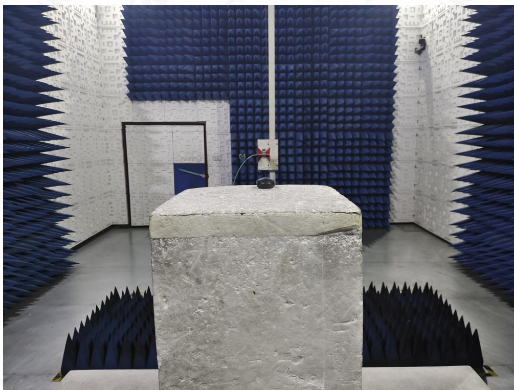
RADIATED EMISSION TEST SETUP ABOVE 1GHz
