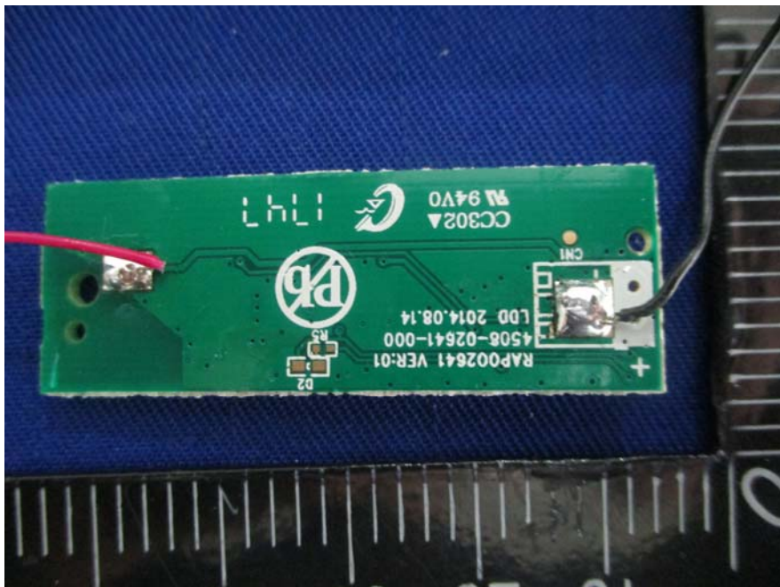
EUT – Main Board Bottom View
