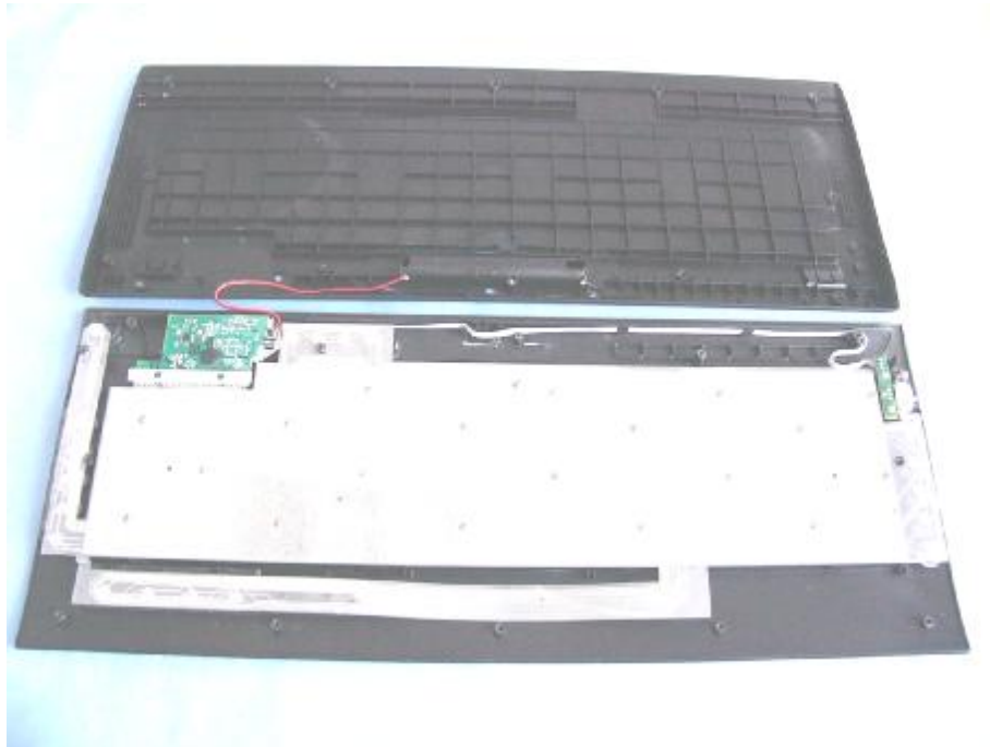
Main board component side
